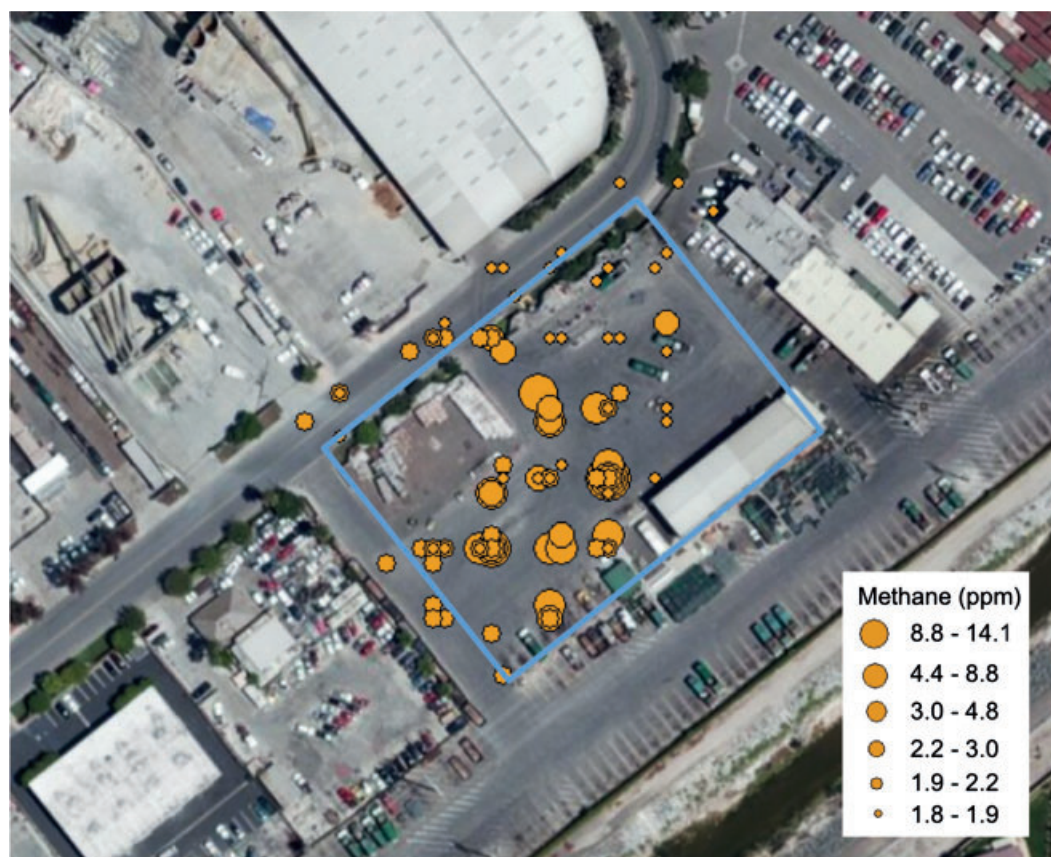
Figure 2. Methane measurements at a compressed natural gas vehicle fueling station in Irvine, California. Fueling station outlined in blue.
